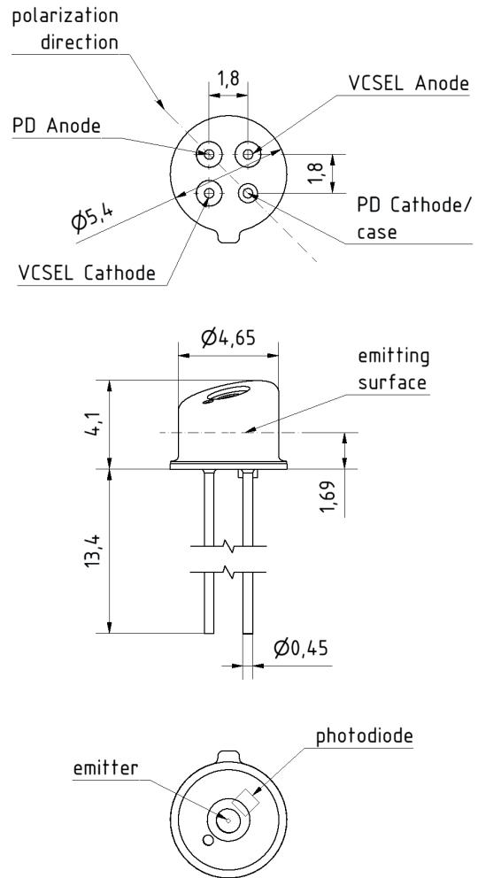
Placement accuracy  $\pm 150 \mu\text{m}$  VCSEL eye to centre of TO cap.
