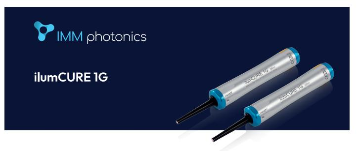
The UV handheld lighting device ilumCURE 1G by IMM Photonics is an UV light source with a central wavelength of 365 nm or 405 nm. It serves as mobile UV light source for the curing of UV adhesives.
