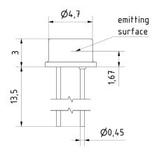
Placement accuracy ±150um VCSEL eye to centre of TO cap.
