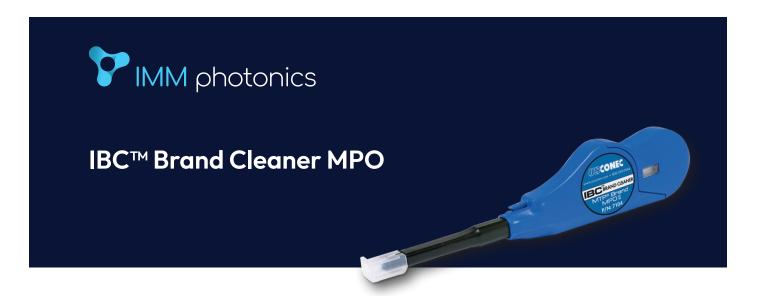
Patented fiber optic cleaner (US Conec) for cleaning MPO connectors. The cleaning pin turns while the cleaning band is drawn over the fiber end surface. This ensures that the fiber end surface is left clean after a single cleaning operation.
