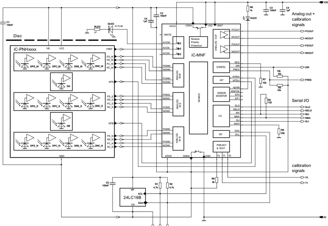
Figure 7: Application example of absolute encoder circuit.
