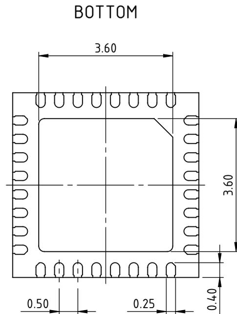
All dimensions given in mm. General Tolerances of form and position according to JEDEC MO-220.
