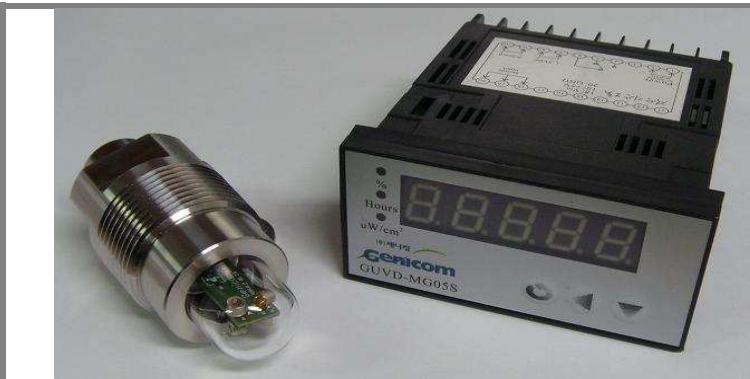
Fig. 1 UV Radiometer 5.0 (Size of Display : 96 × 48 × 112mm 3 )
