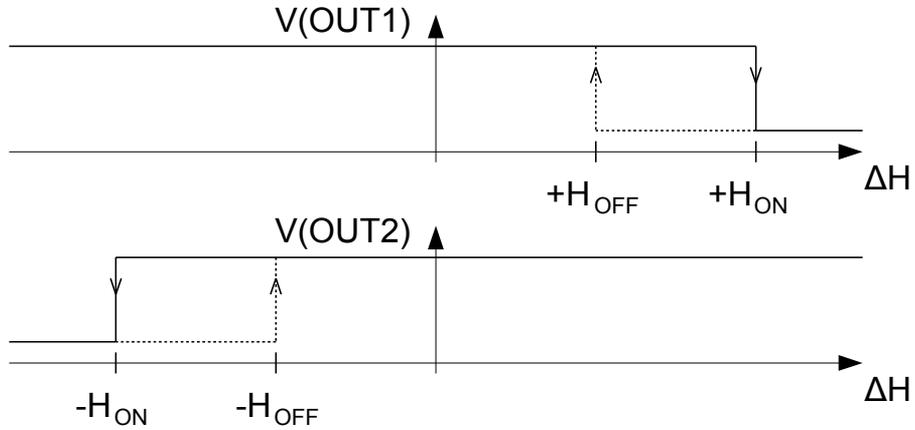
Figure 1: Switching outputs
