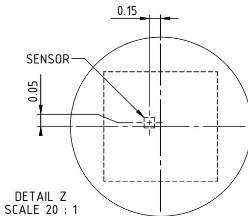
All dimensions given in mm. Tolerances of form and position according to JEDEC MO-229.
